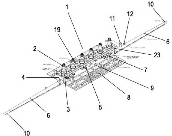
The present invention relates to a vertical branch inline manifold system. In particular the invention relates to a vertical branch inline manifold system for installation on a pipeline conveying hydrocarbon fluids along the seabed.
