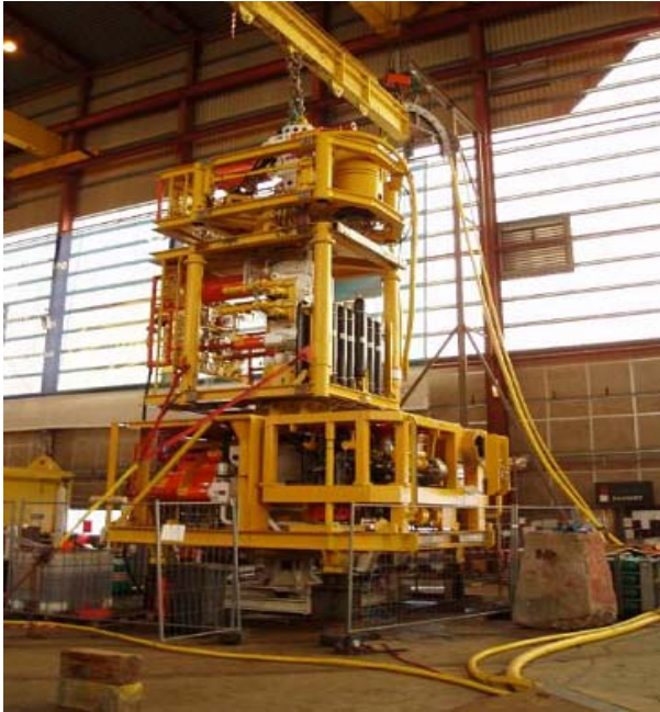
Fig. 11 LRP and EDP stacked on top of the Xmas tree system
