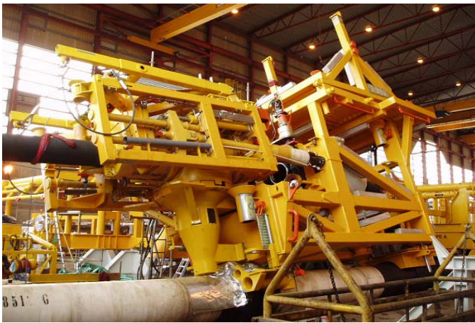
Fig. 16 In-line tee during testing
