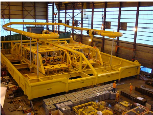
Fig. 19 Testing of PLET modules and pig loop on dummy PLET bottom structure
